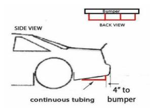
**3.4 FUEL LINES:** All fuel lines must be placed in a safe manner in the car. Mandatory fuel line safety valve OBERG SV-0828 or SRI Performance FPF-FSV must be used/installed as fuel exits the cell also check valve on vent required. Fuel filters mounted at rear of chassis must be located towards the center of the car. No plastic or glass filters permitted. Fuel must travel from the fuel cell to the carburetor and cannot pass into any performance enhancing devices.
